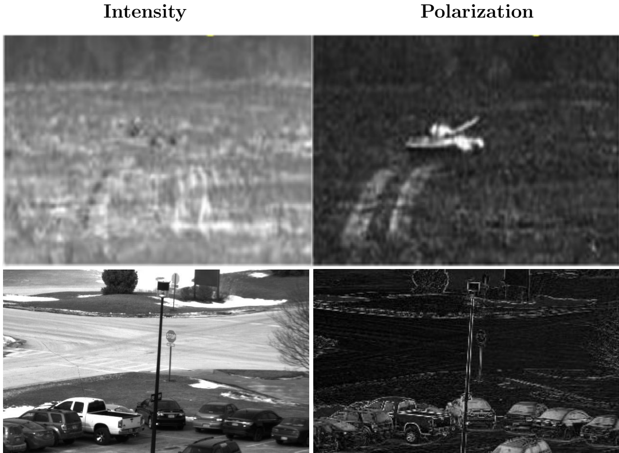
Figure 2. a) Tank in thermal equilibrium, imaged with an infrared camera in intensity and degree of linear polarization (courtesy: David Cenault, Polaris). b) Cars imaged with a microgrid polarizer focal-plane array. In degree of linear polarization only the windshields stand out (courtesy: Dmitry Vorobiev).
